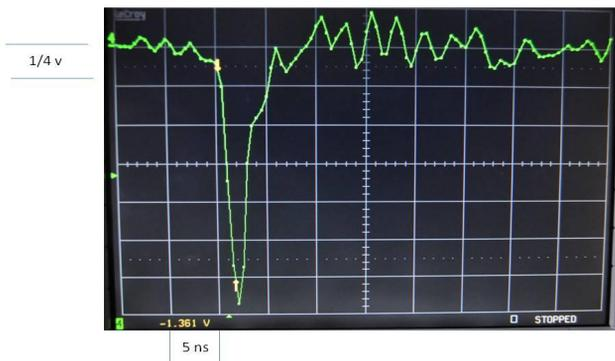
Figure 5: Typical PDP pulse rise time and duration.
