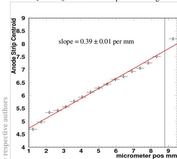
Figure 9. Position resolution beta scan measurements.
