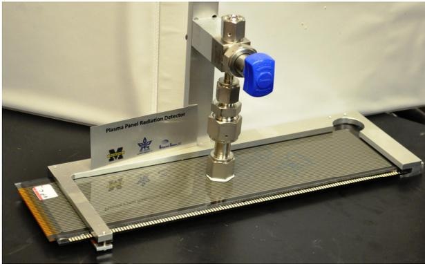
Figure 3: Modified-PDP test panel.
