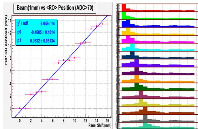
Figure 10: Proton beam position scan with 1 mm aperture.
