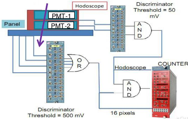
Figure 4: Triple coincidence measurement setup.
