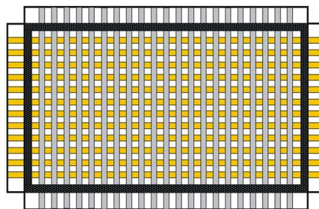
Figure 1: Columnar-discharge, modified-PDP electrode structure. Front cathodes are gray; perimeter seal is black.
