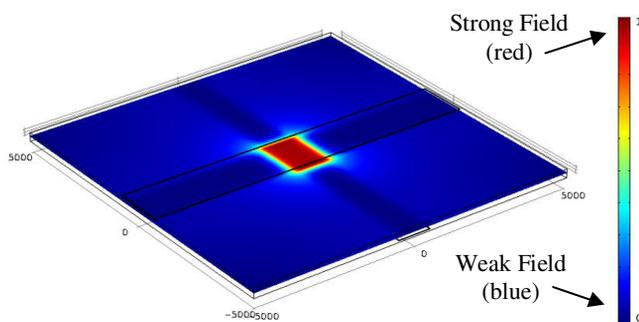
Figure 2: COMSOL simulation of normalized electric field strength inside a PDP single cell.
